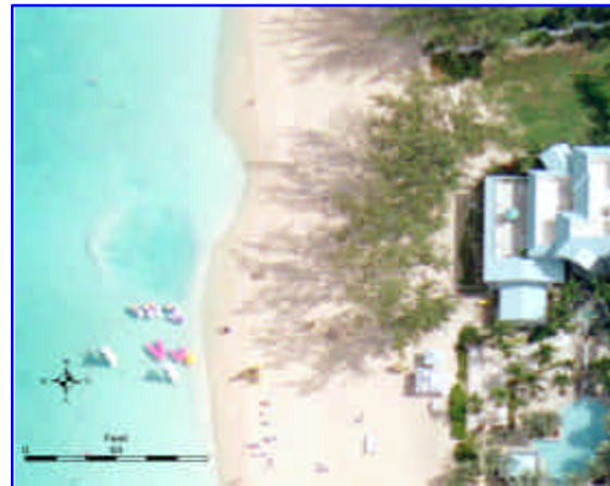
Figure 15: Evidence of local beach erosion hotspots from repeated boat landings.
